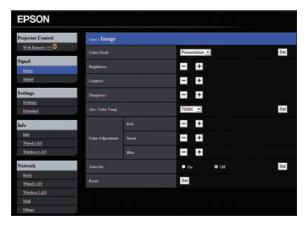
From the Projector Control menu, select **Web Remote**. Use the on-screen buttons to operate the projector, as you would using the remote control.
